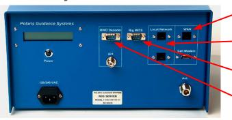
Connect an Ethernet cable between the WAN connector and your Internet
