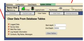
**Step 5 Well information:** Select *Configuration* from the top menu bar and enter the new well information. Press the *Save Changes* button when completed
